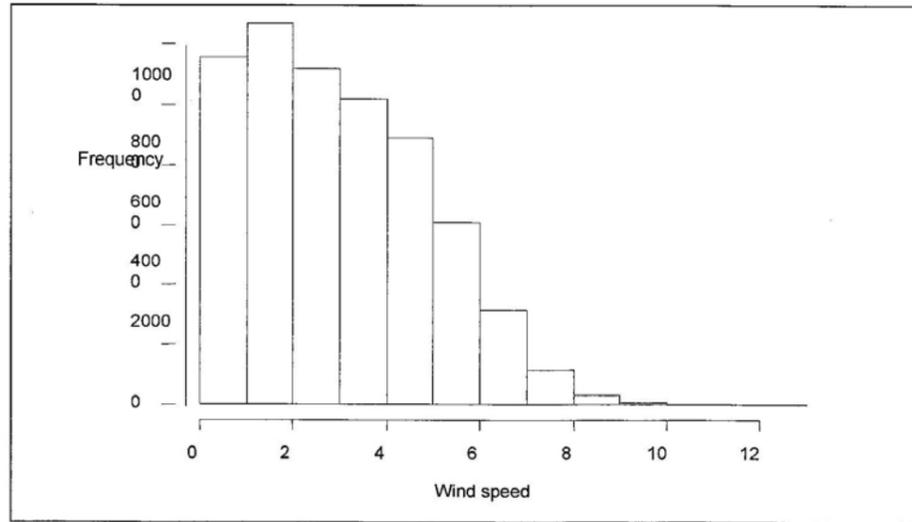
Figure 1: Frequency distribution of wind speed at site A at 10 metre height
