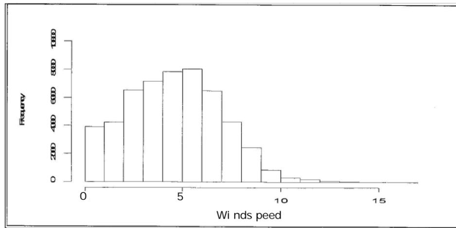
**Figure 7: Frequency distribution of wind speed at site B at 30 metres height**
