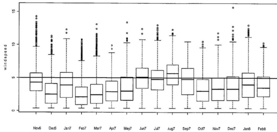
Figure 5: Monthly comparison of wind speed at 30 metre height at site A
