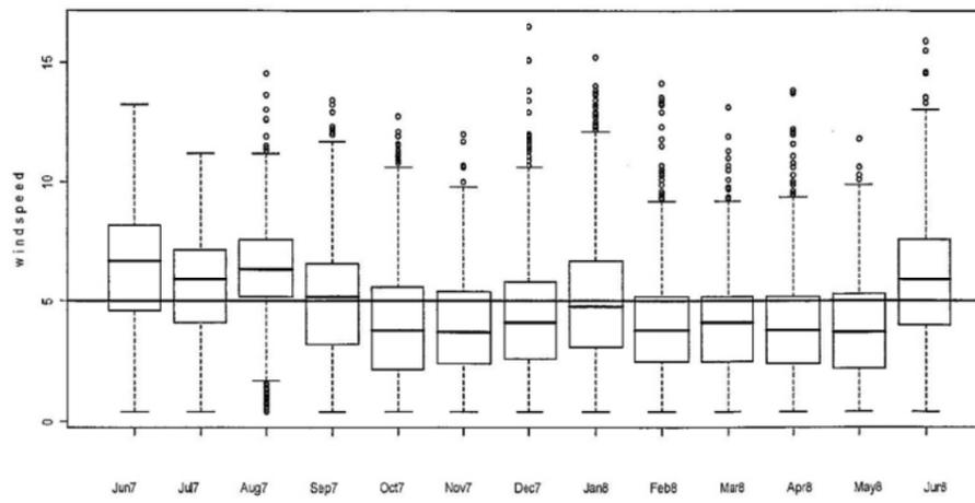
Figure 9: Monthly comparison of wind speed at 30 metre height at site B
